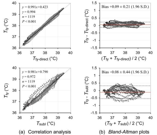
Fig. 3 Analytical results of comparative evaluation test. (a) Relationship between the direct tympanic temperature ( $T_{ty-direct}$ ) and the tympanic temperature measured by the present system ( $T_{ty}$ ), and that between the sublingual temperature ( $T_{subl}$ ) and  $T_{ty}$ , and (b) their *Bland-Altman* plots.
