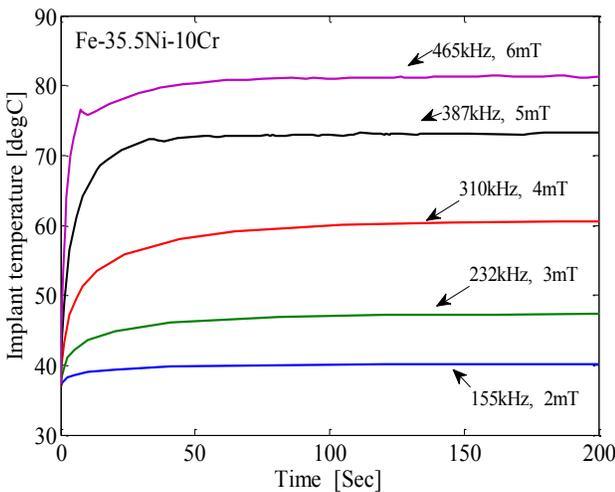
Fig. 10. Temperature characteristics of magnetic shunt steel.
