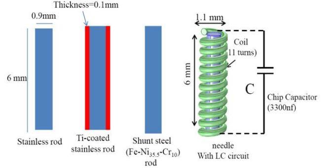
Fig. 3. Implant configurations with aspect ratio around 6.
