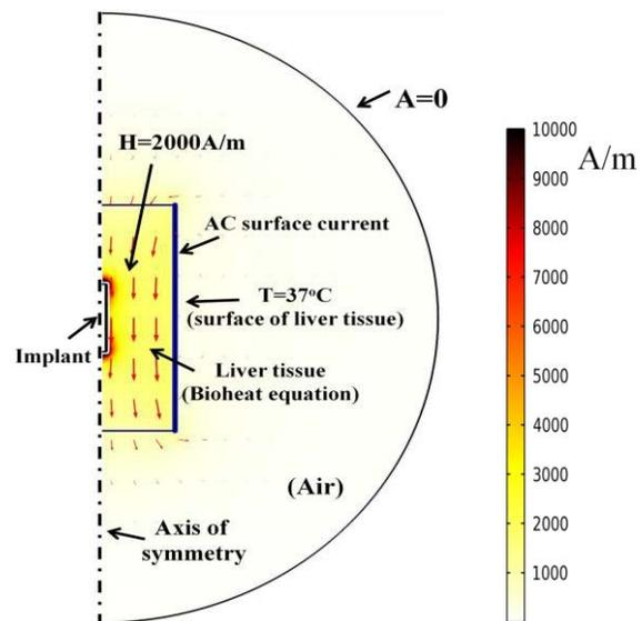
Fig. 1. Two-dimensional model of the heating problem.
