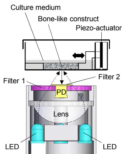
Figure 2 Configuration of the optical device for monitoring  $iCa^{2+}$  responses of osteoblasts under dynamic loading conditions accompanied by substrate deformation. Four LEDs excite the  $Ca^{2+}$  fluorescence indicator Fluo-4 in osteoblasts by irradiating a construct subjected to dynamic loading with a light of 488-nm wavelength. Fluorescent light of 518-nm wavelength emitted by Fluo-4 is detected by a PD positioned at the center of the device.
