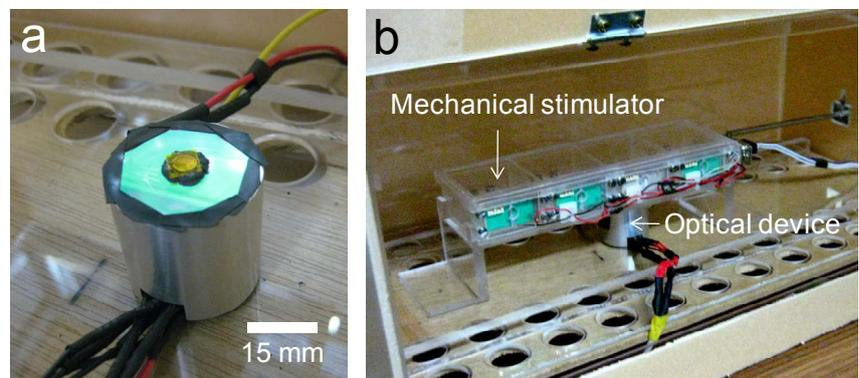
Figure 3 Photographs of the optical device. (a) Overall appearance of the device, (b) The device installed underneath the mechanical stimulator in a homeothermal container at 37°C.
