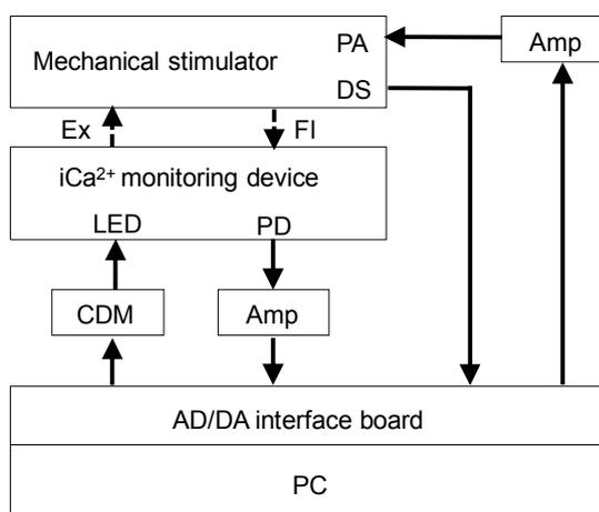
Figure 5 Configuration of the experimental system. PA: Piezoelectric actuator, DS: Displacement sensor, Ex: Excitation light, Fl: Fluorescent light, CDM: Current-drive module, Amp: Amplifier, PC: Personal computer.
