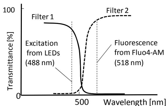
Figure 4 Transmittance properties of the optical filters 1 and 2 selected for Fluo-4. Light from LEDs (wavelength of approximately  $< 500$  nm) passes through filter 1 while light from a construct (wavelength of approximately  $> 500$  nm) passes through filter 2. The wavelength of the excitation light from the LEDs is 488 nm and that of the fluorescent light emitted by Fluo-4 is 518 nm.
