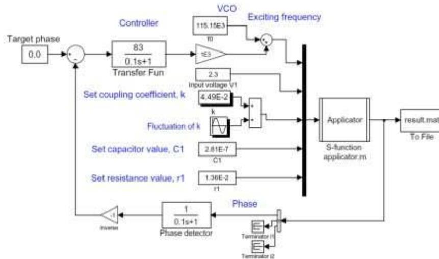
**Fig. 9** Simulation program of control and applicator by MATLAB/Simulink.
