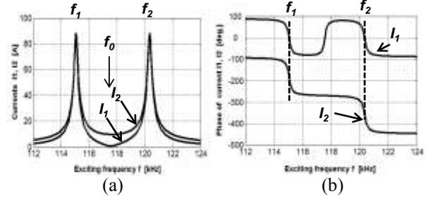
**Fig. 5** Characteristics of exciting  $I_1$  and induced currents  $I_2$ . (a) Amplitude. (b) Phase differences to input voltage.
