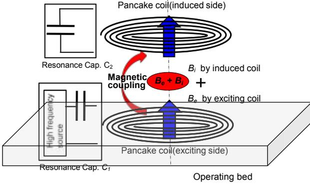
**Fig. 2** Applicator with wireless transmission system.
