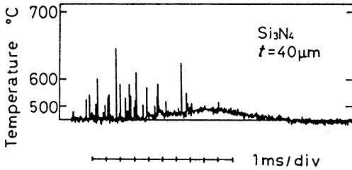
Fig. 7 Output wave of grinding temperature in surface layer of Si 3 N 4
