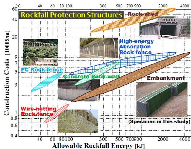
Fig. 1 Construction costs for rockfall protection structures
