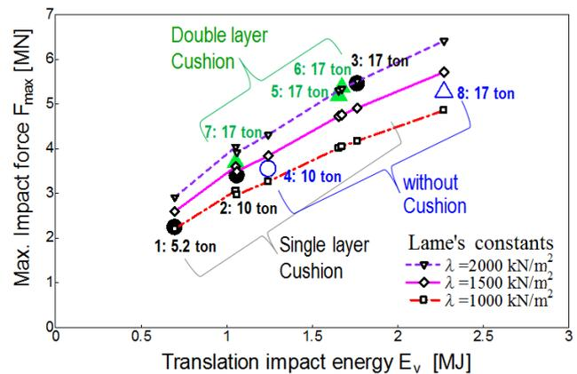
Fig. 12 Impact forces by prediction and measurement
