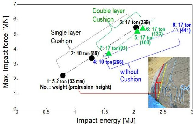
Fig. 13 Relationship between impact energy and force
