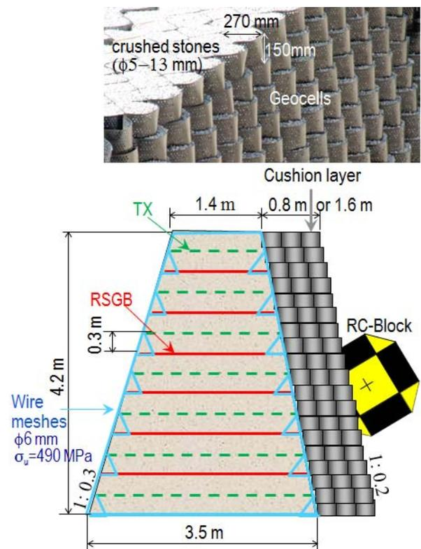
Fig. 3 Geometric scheme of embankment & cushion layer
