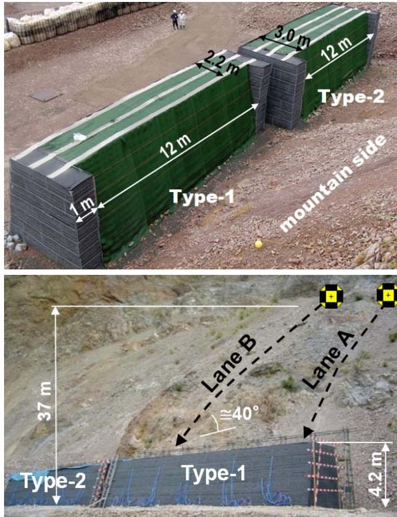
Fig. 2 Features of embankments and rock-slope lanes
