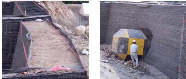
Fig. 11 After the impact of test No. 8
