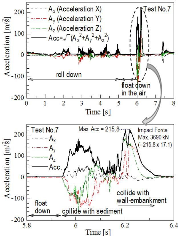
Fig. 9 Example of acceleration of RC block
