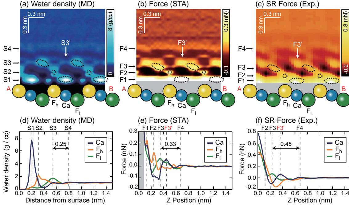
**Fig. 3**  $z$  cross sections of the (a)  $\rho(\mathbf{r})$ , (b)  $F_{STA}(\mathbf{r})$  and (c)  $F_{exp}(\mathbf{r})$  images.  $z$  profiles of the (d)  $\rho(\mathbf{r})$ , (e)  $F_{STA}(\mathbf{r})$  and (f)  $F_{exp}(\mathbf{r})$  images over Ca,  $F_h$  and  $F_l$  sites.
