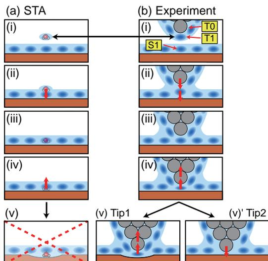
**Fig. 5** Schematic models showing relationship between a tip position and a measured force in (a) the STA model and (b) a real experiment.
