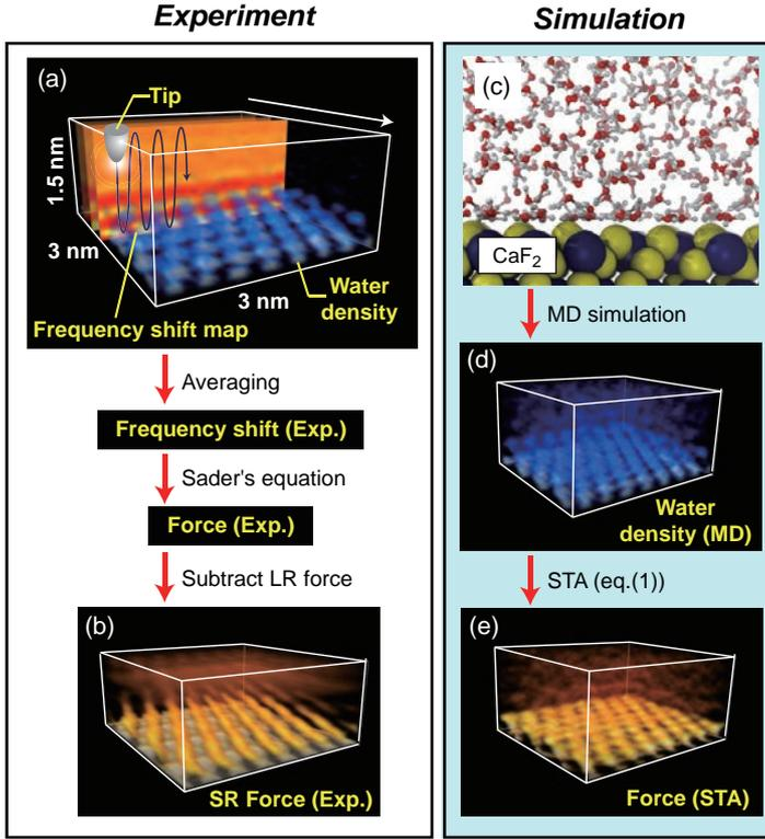
**Fig. 2** Outline of the methods used for obtaining 3D  $F(\mathbf{r})$  maps at a fluorite(111)-water interface by experiment and simulation. (a) Measurement of 3D  $\Delta f$  distribution. (b) 3D SR  $F(\mathbf{r})$  distribution converted from (a). (c) Snapshot of the MD simulation model. (d) 3D  $\rho(\mathbf{r})$  distribution obtained by the MD simulation. (e) 3D  $F(\mathbf{r})$  distribution calculated from (b) using the STA model.
