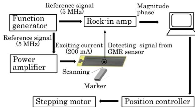
Fig. 9 Measurement system.
