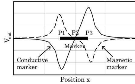
**Fig. 2** Magnitude of  $B_x$  signal considering phase.
