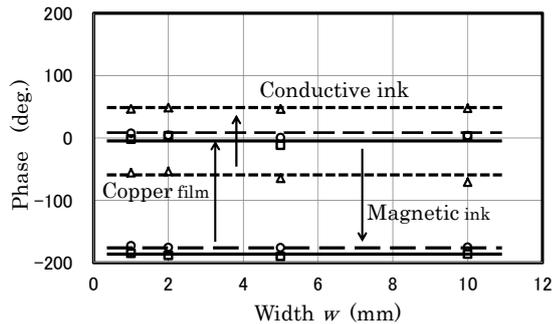
**Fig. 12** Phase shift vs. width of markers with different materials.
