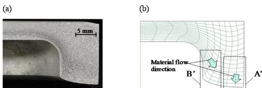
Fig. 9. Cross-section in case of free forging without the back-pressure load application; (a) Formed part; (b) Simulation.
