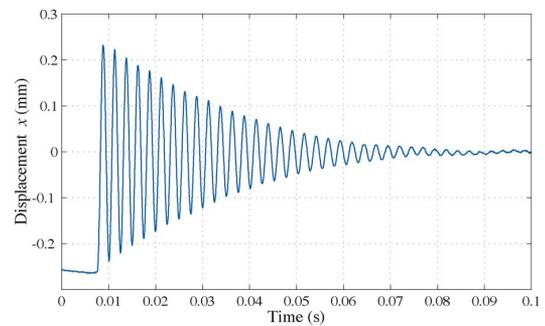
Fig. 6. Displacement at free vibration ( $fr = 392$  Hz).
