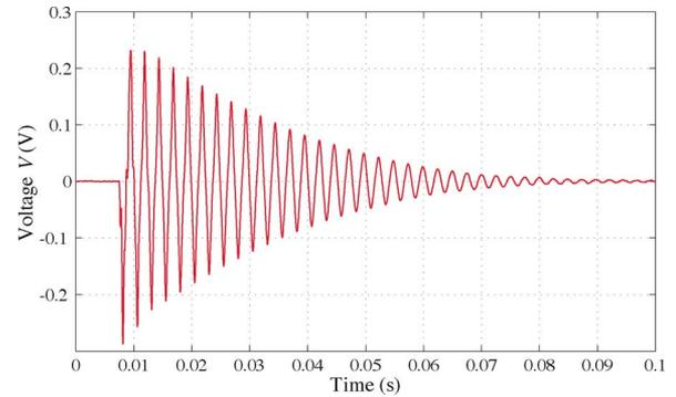
Fig. 5. Generated voltage at free vibration ( $fr = 392$  Hz).
