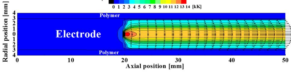
Fig. 3. Calculated two dimensional temperature and gas flow distributions in the PA6 ablated arc.
