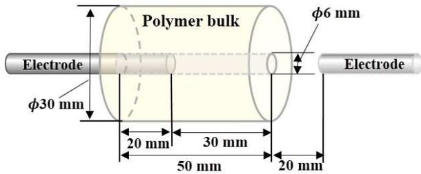
Fig. 1. Schematics of the calculation target imaging the arc device.
