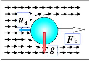
Fig. 6. Exerted drag force and gravity on a spallation particle flying in gas flow.
