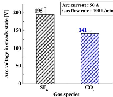
Fig. 10. Averaged arc voltage measured in steady state.
