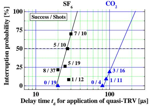
Fig. 8. Dependence of successful interruption probability on delay time  $t_d$  for quasi-TRV application, in cases of the nozzle with holes covered by plates.
