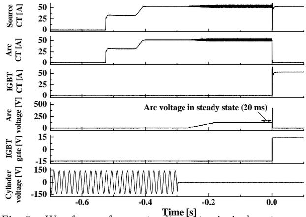
Fig. 6. Waveforms of current-voltage at principal parts.
