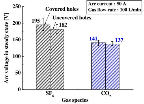
Fig. 14. Averaged arc voltage measured in steady state.
