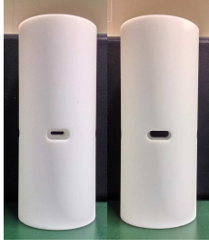
Fig. 11. The nozzle with uncovered holes.
