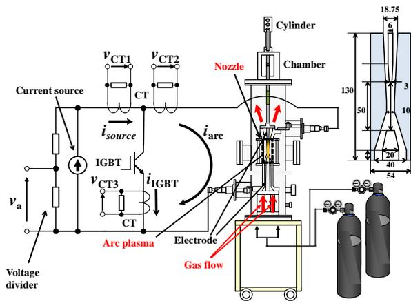
Fig. 4. Experimental setup for gas-blast arc experiment.
