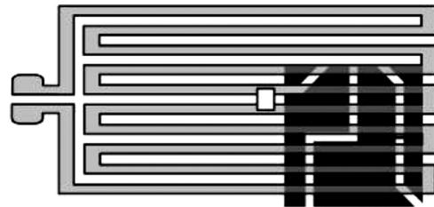
Fig. 1. A Meander-type coil is shown above a PCB while a GMR sensor is set at the midpoint of the coil.
