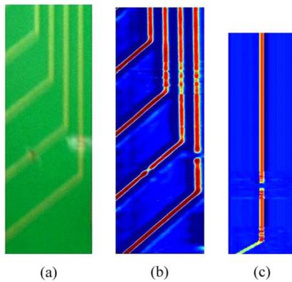
Fig. 5. (a) Photo of a real PCB. (b) Image of the PCB obtained by experiment after applying image processing technique. (c) Image obtained by base-model method for a small part of the PCB.
