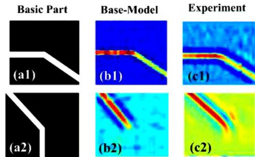
Fig. 4. (a1), (a2) Basic parts obtained after disassembling. (b1), (b2) Base-model results of scanning simulation based on 3D FEM analysis. (c1), (c2) Experimental results of the same pattern PCB, notice that the scanning direction is from left to right in the horizontal direction.
