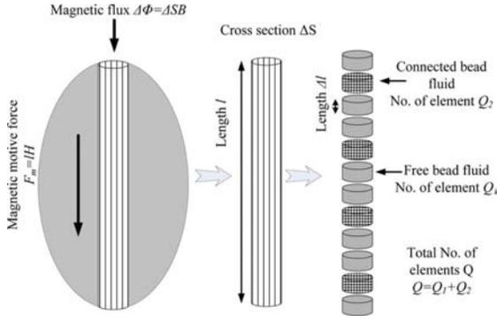
Fig. 2. Magnetic path and permeability of mixed fluids.
