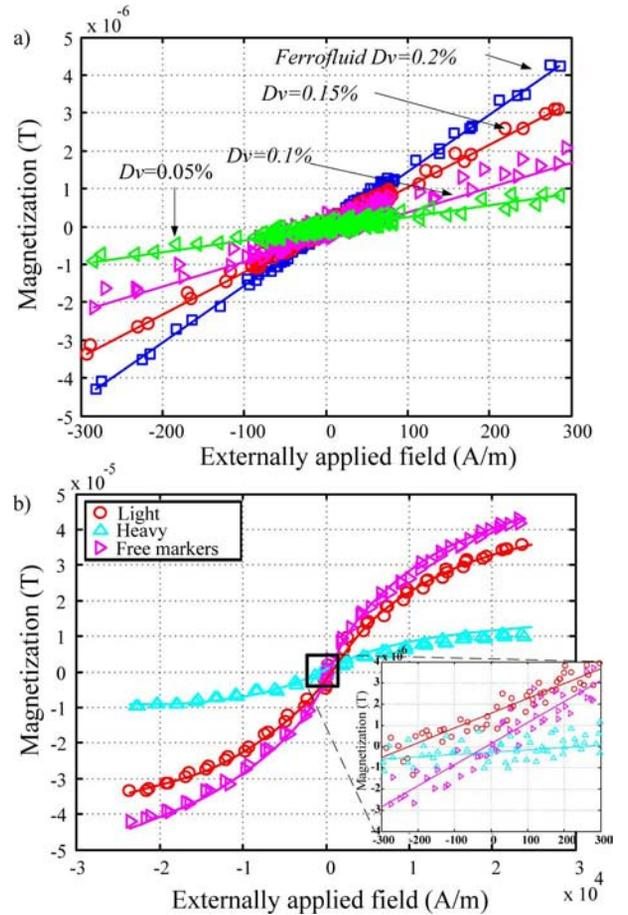
Fig. 6. VSM measurement. (a) Dilution influence. (b) Characteristics of centrifuged magnetic markers combined with polymer beads and free markers.
