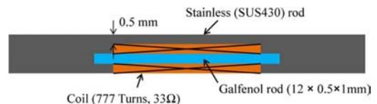
Fig. 1. Structure of the unimorph vibration energy harvester.
