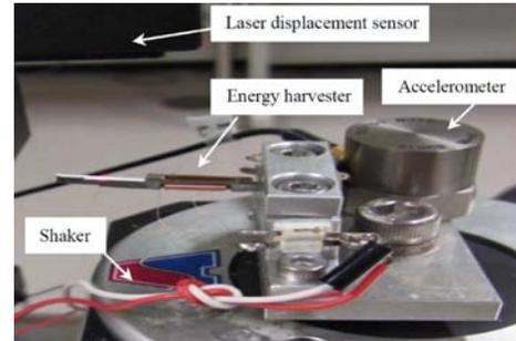
Fig. 9. Measurement setup.
