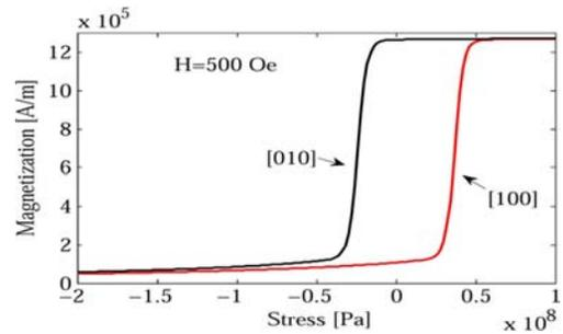
Fig. 3. Magnetization curves under uniaxial mechanical stress.
