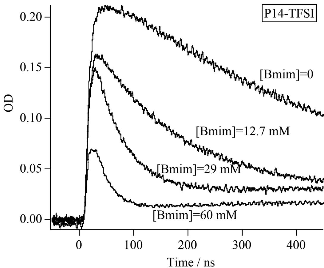
Fig. 4. Kinetics of the reaction of electron with Bmim in P14-TFSI observed at 700 nm after 248-nm excitation.
