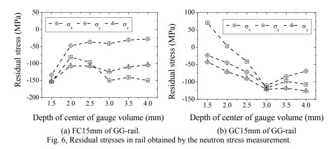
It is also seen that the normal stress components have similar values each other except a part of  $\sigma_z$ . It is not clear why the residual stress state in the rail was a hydrostatic. More research needs to be conducted in order to answer that question. However, the fact that a compressive stress layer surrounding rail head with about 10mm thickness restricts inside deformation from three sides may be one of the reasons.
