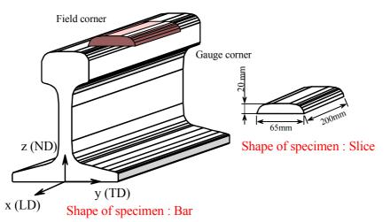
Fig. 1, Sampling of rail specimen used for the neutron stress measurement.
