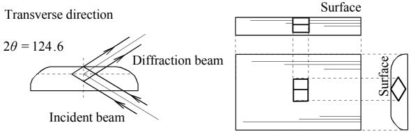
Fig. 4, Schematic of gauge volume for neutron stress measurement.
