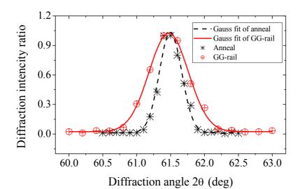
Fig. 5, Example of diffraction pattern obtained from rail at point P1 (z=2.0 mm) in LD direction.
