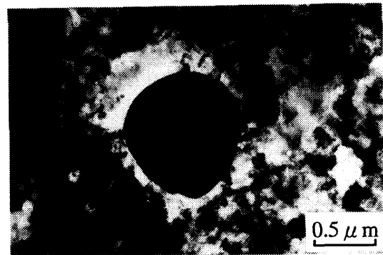
Fig.3 Nucleation of recrystallization at a Fe 3 P particle.
