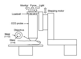
Fig.1 The diagrammatic representation of the system assembly. The capillaroscopy is composed of a CCD video-probe and a contact-type objective lens with a coaxial epi-illumination. The CCD probe was attached to a one-way movable actuator with a force transducer to visualize the dynamic responses of the dermal capillary flow being compressed at the skin surface.
