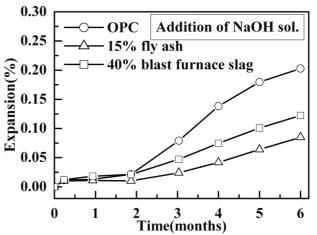
Figure 15. Expansion behaviors of concretes using recycled coarse aggregate and river sand with 15 % fly ash and 40 % blast furnace slag.
