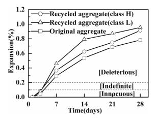
Figure 11. Expansion behaviors of mortars using recycled aggregate and original aggregate (ASTM C1260).
