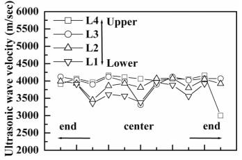
Figure 5. Change in ultrasonic wave velocity of pillow beam.
