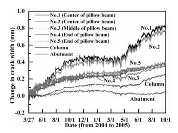
Figure 7. Variations in crack width of RC pier and abutment.
