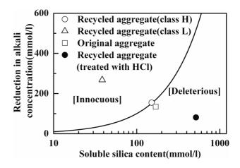
Figure 9. Results of chemical method of recycled aggregate and original aggregate (JIS A1145).
