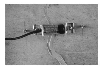
Figure 6. Sensor attached across cracks on surface of pillow beam.
