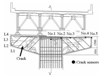
Figure 4. Schematic diagram of cracking of pillow beam.
