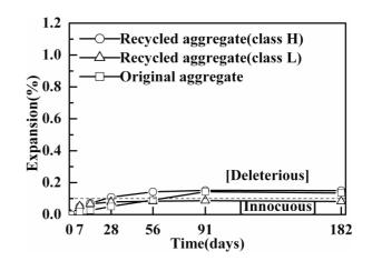
Figure 10. Expansion behaviors of mortars using recycled aggregate and original aggregate (JIS A1146).
