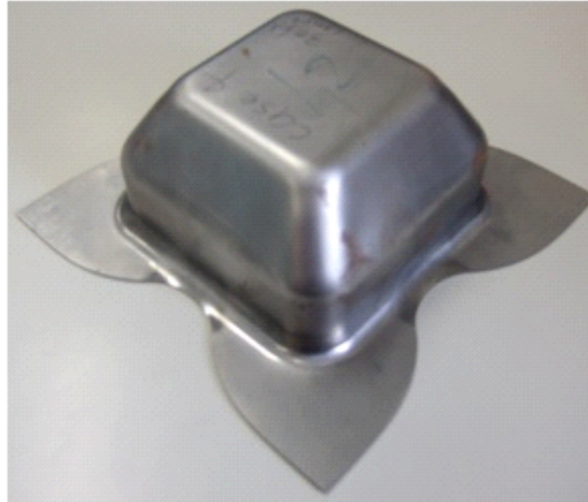
Fig.2(a) Formed part obtained in the experiment performed with a constant BHF of 100[kN]
