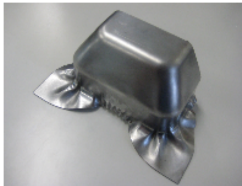
Fig.8 Wrinkling predicted in the experimental test performed with a constant BHF of 20 [kN]
