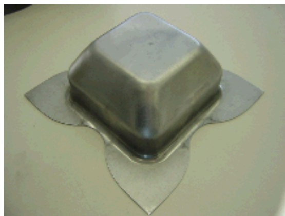
Fig. 15 The square cup deep drawing in the experiment (Initial BHF=20[kN])
