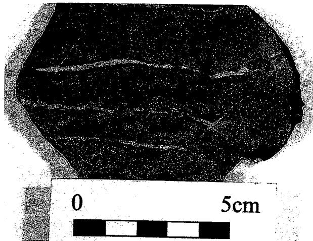
Fig. 2. Photograph of the lherzolite xenolith cut by anastomosing quartz diorite veins (white). Foliation is defined by dark lenticular aggregates of spinel and pyroxenes.
