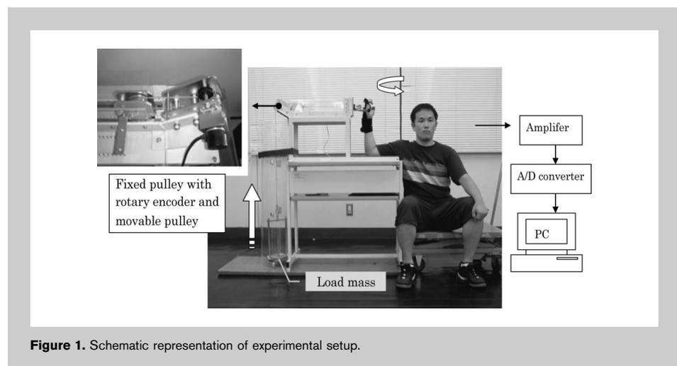
Figure 1. Schematic representation of experimental setup.
