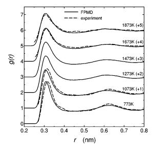
FIG. 7. Comparison of the radial distribution function, g(r), of liquid Sn between the present experiment (open circle) and the first-principle molecular-dynamics (FPMD) simulation (solid line).
