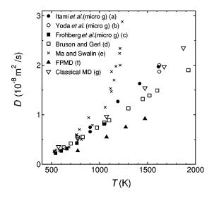
FIG. 15. The self-diffusion coefficient, *D*, of liquid Sn as a function of temperature, *T*; microgravity experiments: (a) Itami *et al.*, (Ref. 11), (b) Yoda *et al.* (Ref. 12), and (c) Frohberg *et al.* (Refs. 9 and 10); experiments on the ground: (d) Bruson and Gerl (Ref. 62) and (e) Ma and Swallin (Ref. 61); molecular dynamics (MD): (f) the present first-principle MD (FPMD), and (g) the present classical MD.
