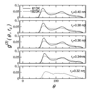
FIG. 9. The angle,  $\theta$ , dependence of angle distribution function,  $g^{(3)}(\theta, r_c)$ , of liquid Pb in spheres with cutoff radii  $r_c$ 's.
