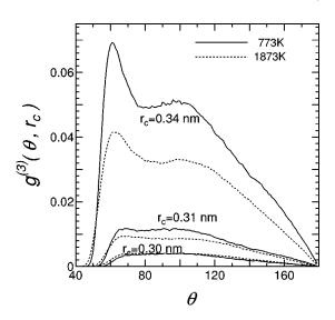
FIG. 8. The angle,  $\theta$ , dependence of angle distribution function,  $g^{(3)}(\theta, r_c)$ , of liquid Sn in spheres with cutoff radii  $r_c$ 's.
