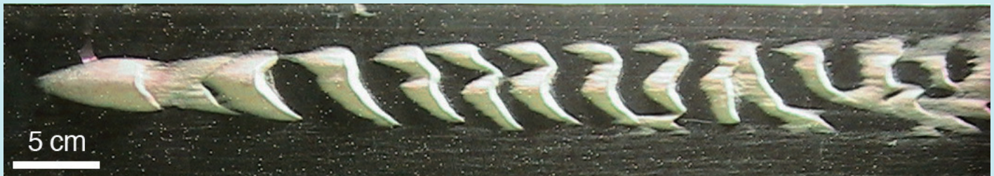
Fig. 2. Small (ripple-sized) barchan trains formed in a flume. The flow and barchans run from left to right.
