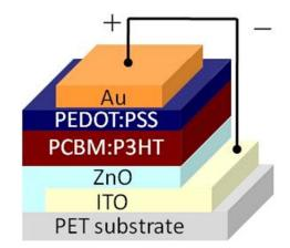
Figure 1 Device structure of the inverted polymer solar cells.
