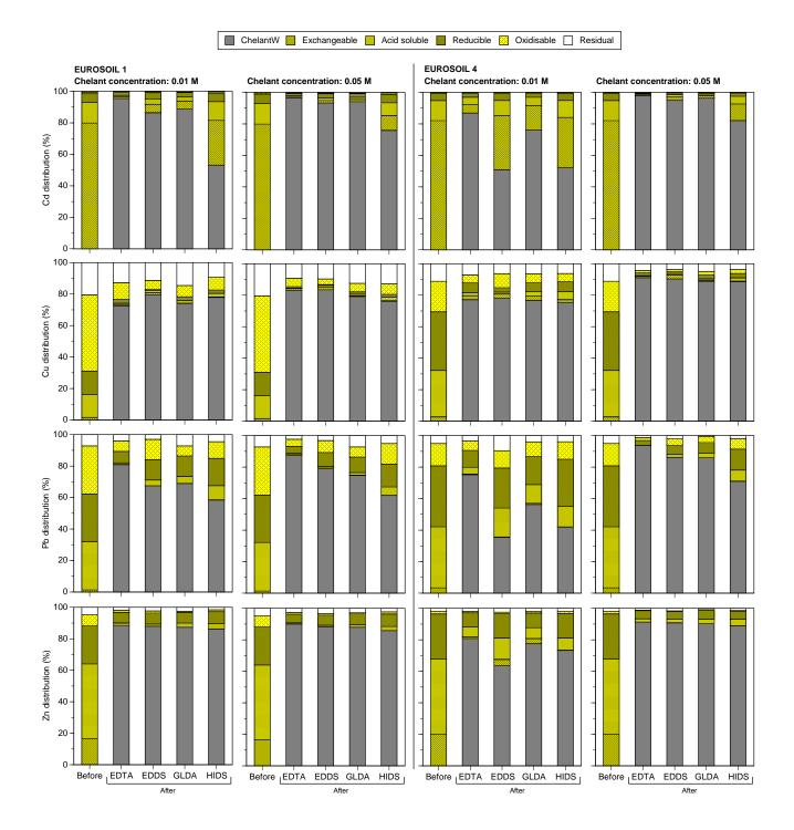
**Figure 4.** Comparative distribution of the toxic metals (Cd, Cu, Pb and Zn) in the solid phase of Eurosoil 1 and Eurosoil 4 before and after the treatment with different chelants (EDTA, EDDS, GLDA and HIDS; pH = 7).
