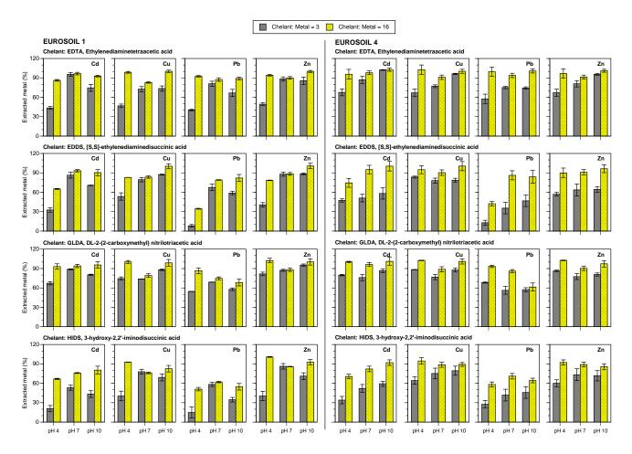
**Figure 1.** Comparative extraction (%) of the toxic metals (Cd, Cu, Pb and Zn) at varying chelant-tometal molar ratios (3 and 16) from the Eurosoil 1 and Eurosoil 4 with different chelants (EDTA, EDDS, GLDA and HIDS) at controlled solution pH.
