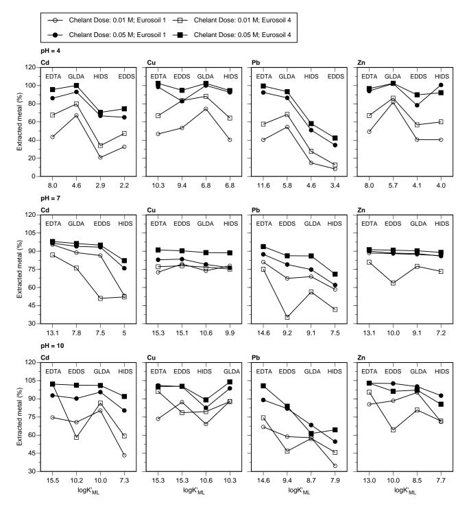
**Figure 3.** Extraction selectivity of the biodegradable chelants (EDDS, GLDA and HIDS) towards the toxic metals (Cd, Cu, Pb and Zn) in terms of the order (largest to smallest) of conditional metal-chelant stability constants ( $\log K'_{ML}$ ) from the Eurosoil 1 and Eurosoil 4.
