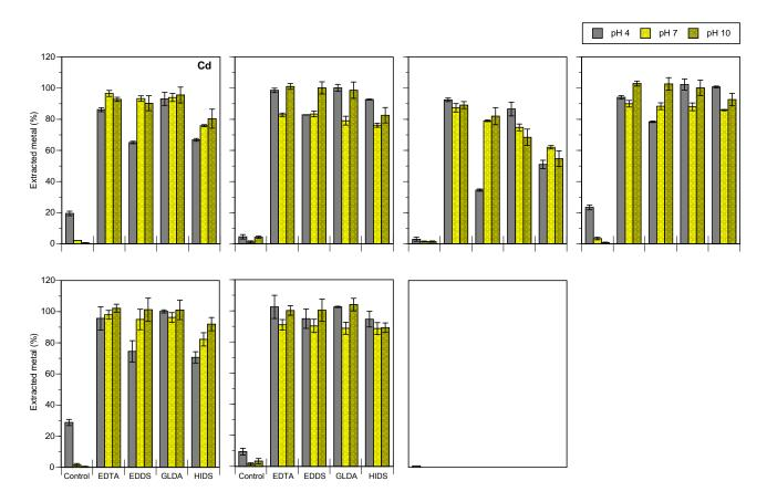
**Figure 2.** Comparative extraction rate (%) of the toxic metals (Cd, Cu, Pb and Zn) at varying pH conditions (4, 7 and 10) from the Eurosoil 1 and Eurosoil 4 with different chelants (EDTA, EDDS, GLDA and HIDS; 0.05 M).
