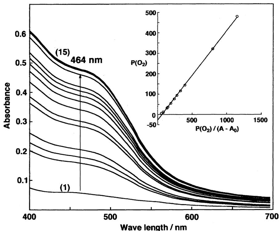
Fig. 6. Spectral change of **9** at various partial dioxygen pressures in  $\text{CH}_3\text{CN}$  at  $20^\circ\text{C}$ : (1) 0 Torr, (2) 5.5 Torr, (3) 10 Torr, (4) 12 Torr, (5) 31 Torr, (6) 36 Torr, (7) 54 Torr, (8) 76 Torr, (9) 93 Torr, (10) 115 Torr, (11) 143 Torr, (12) 321 Torr, (13) 480 Torr, (14) 524 Torr, (15) 563 Torr.
