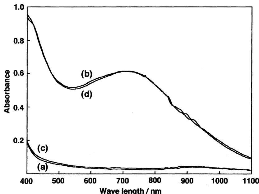
Fig. 3. Electronic spectral change of **1** in CH<sub>2</sub>Cl<sub>2</sub> under O<sub>2</sub>.
