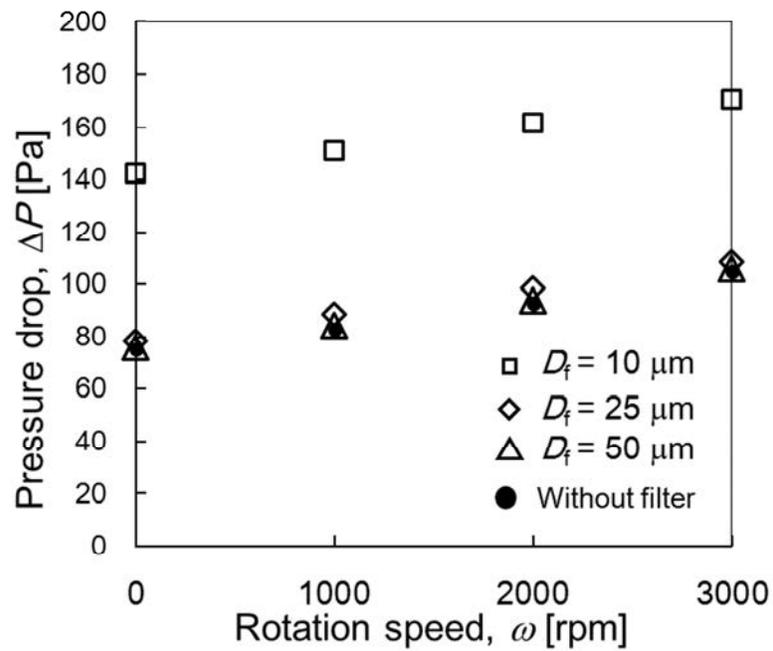
FIG.6. Pressure drops of centrifugal filter consisting of fibers with different diameters as a function of rotation speed at a fixed filtration velocity,  $u_0$ , of  $5.0 \text{ cm s}^{-1}$ .
