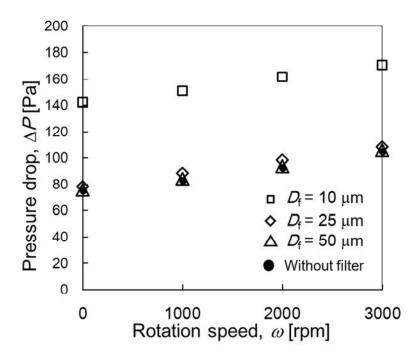
FIG.6. Pressure drops of centrifugal filter consisting of fibers with different diameters as a function of rotation speed at a fixed filtration velocity,  $u_0$ , of 5.0 cm s<sup>-1</sup>.
