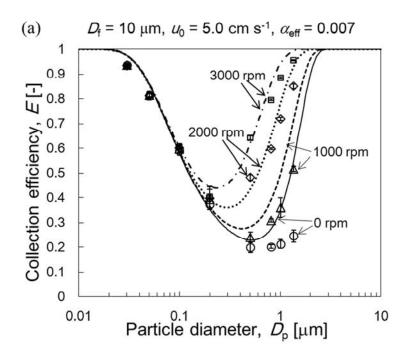
FIG.3. Collection efficiencies of centrifugal filter against particle diameter ( $u_0 = 5.0 \text{ cm s}^{-1}$ ,  $D_f = 10$ , 25, 50  $\mu m$ ). (lines are predicted by Eq. (1), and symbols are experimental data) 793x595mm (96 x 96 DPI)
