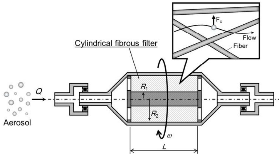
FIG.1. Basic concept of aerosol collection by centrifugal filter.
