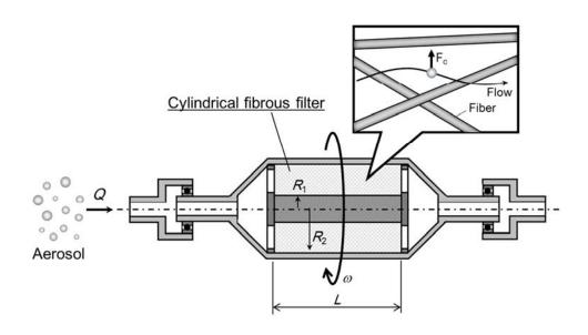
FIG.1. Basic concept of aerosol collection by centrifugal filter. 793x595mm (96 x 96 DPI)
