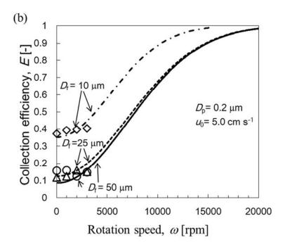
FIG.4. Collection efficiency of centrifugal filter against rotation speed at the fixed filtration velocity,  $u_0$ , of 5.0 cm s $^{-1}$ . (lines are predicted by Eq. (1), and symbols are experimental data) 793x595mm (96 x 96 DPI)
