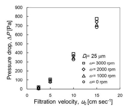
FIG.5. Pressure drop of centrifugal filter against the filtration velocity with the rotation speed as a parameter. 254x190mm~(300~x~300~DPI)
