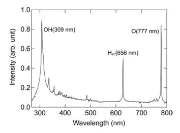
Fig. 2. Optical emission spectrum of the plasma.
