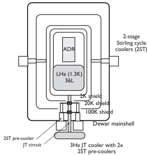
Figure 1: Design concept of the SXS cooling system.
