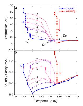
Fig. 2. (Color online) Attenuation and velocity of <sup>4</sup>He in 97.0% porous aerogel. The curves labeled as a-f are hysteresis loops with the lowest temperatures successively approaching the onset of freezing at  $T_f = 1.795$  K.
