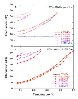
Fig. 4. (Color online) Attenuations of 10 MHz ultrasound for (a) pure <sup>4</sup>He and (b) <sup>4</sup>He with 0.16% <sup>3</sup>He in 97.0% porous aerogel at various freezing pressures  $p_f$ . The attenuation of pure liquid <sup>4</sup>He at 2.6 MPa is also shown in (a) for comparison.
