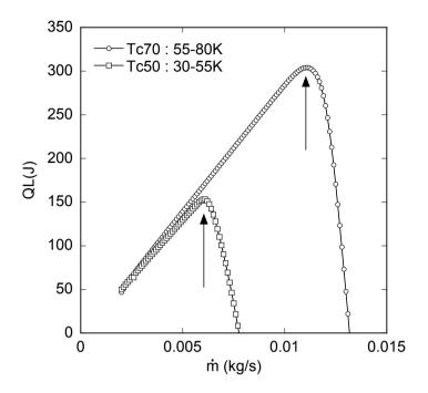
Figure 3: Heat load of AMR using single material of Tc70 and Tc50 as functions of  $\dot{m}$ . The operation temperature span is 25 K for both cases but temperature range is between 80 and 55 K for Tc70 and between 55 and 30 K for Tc50. Arrows represent the optimum  $\dot{m}$ .
