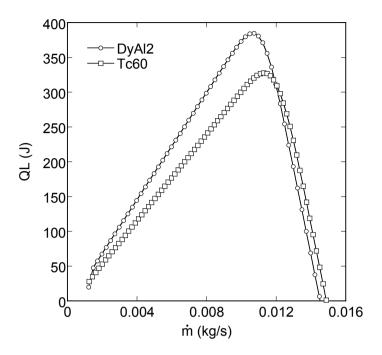
Figure 2: Heat load of AMR using material with Tc60 as a function of  $\dot{m}$ . That using DyAl<sub>2</sub> is also represented for comparison. The operation temperature range is between 77 and 65 K.
