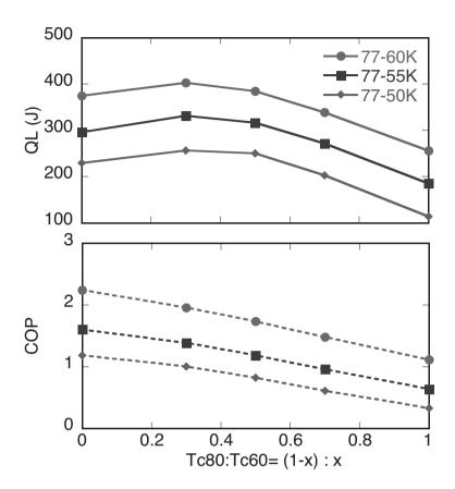
Figure 5: Heat load and COP of two layered AMR with Tc80 and Tc60 as functions of ratio between the two materials. Results for  $T_L = 60$ , 55, and 50 K are shown.  $T_H$  is 77 K.
