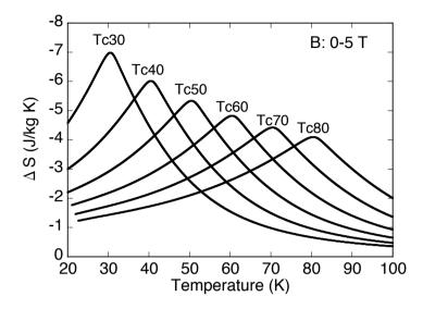
Figure 1: Magnetic entropy change of model materials with various transition temperature  $T_c$  induced by 5 T field, as calculated using mean field theory. Each curve respectively corresponds to  $\Delta S$  of Tc30, Tc40, Tc50, Tc60, Tc70, and Tc80 from low temperature.
