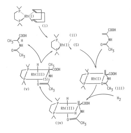
Fig. 4. Cycle of the catalyst for asymmetric hydrogenation.
