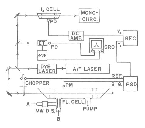
Fig. 1. Schematic of experimental apparatus for laser excitation spectra.
