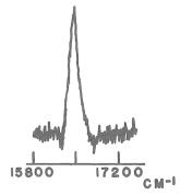
Fig. 8. Absorption spectrum of benzene-h<sub>6</sub> obtained by means of thermal lens technique.
