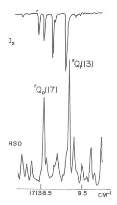
Fig. 2. An example of the excitation spectrum. The  $\tilde{A}^2 A'(004) \leftarrow \tilde{X}^2 A''(000)$  vibronic trasition of HSO is shown in the lower trace. The upper trace is the iodine spectrum recorded for the wavenumber calibration.
