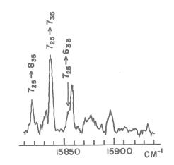
Fig. 4. The fluorescence spectrum of HCF terminating on the  $\tilde{X}^1 A'(010)$  level, observed following the selective excitation to the 7<sub>25</sub> level of the  $\tilde{A}^1 A''(000)$ .
