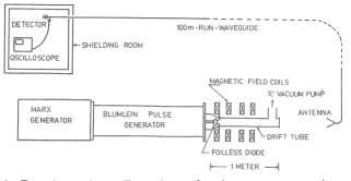
Fig. 1 Experimental configuration of microwave generation. The dispersive line is a 100-m length of X-band waveguide.
