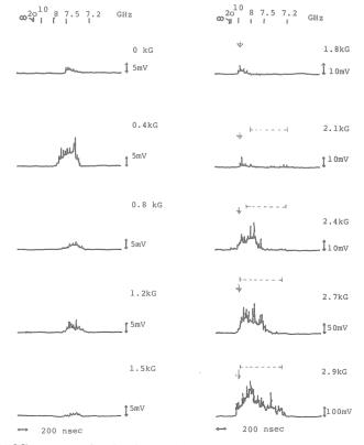
Fig.12 Microwave signals from the rippled field waveguide as a parameter of the guide field.
