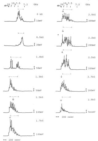
Fig.10 Microwave signals from the smooth metallic waveguide as a parameter of the guide field.
