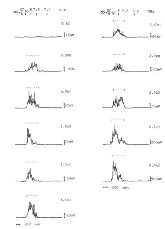
Fig.13 Microwave signals from the dielectric loaded waveguide as a parameter of the guide field.
