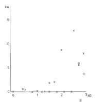
Fig.15 Microwave power as a function of the guide field. Microwave radiation x: from the smooth metallic waveguide, o: from the rippled magnetic field waveguide.
