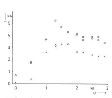
Fig.18 Propating beam currents monitored by the magnetic probes in the drift tube. These currents were picked up at the position 1 (o marked) and 2 (x marked) in Fig. 2.
