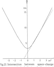
wave (dashed line) and the dielctric loaded waveguide (solid curve).
