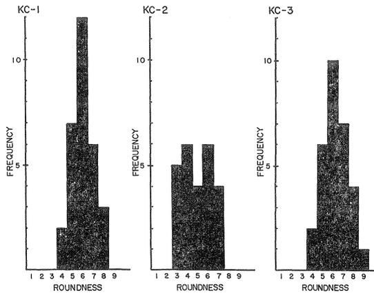
Text-figure 3. Histograms of roundness distribution as measured from 30 gravels at three units of the Kamihirose formation (by KRUMBEIN's silhouette method). KC-1, unit 5; KC-2, unit 13; and KC-3, unit 27.
