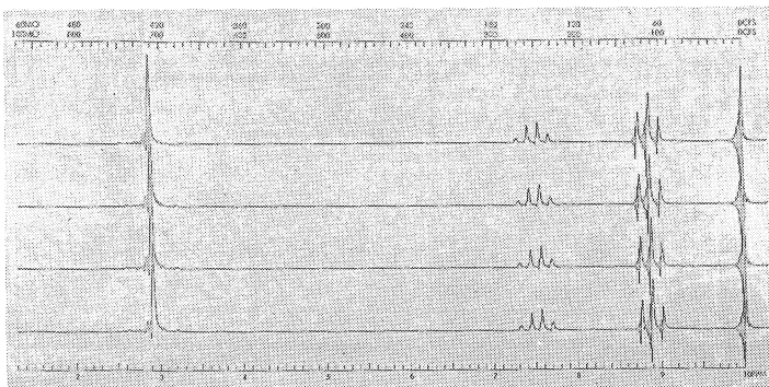
Fig. 3. Reproducibility of spectra for 40 minutes (sample is pure ethylbenzene contained a trace of TMS as an internal standard.)
