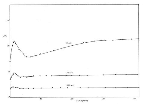
Fig. 15 Capacitance changes during miosture adsorption at the frequencies indicated. (calcined diatomaceous earth)
