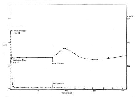
Fig. 6 The result of a simultaneous measurement of the capacitance and conductivity when moisture flow was cut off at the time of peak of the conductivity. (soda lime glass)
