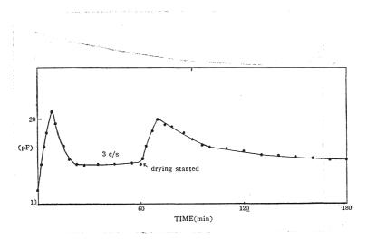
Fig. 2 Capactance changes when a glass plate with adsorbed water was slowly dried. (soda lime glass)
