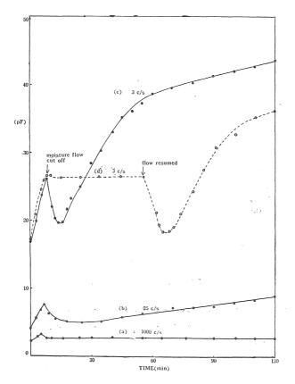
Fig. 7 Capacitance changes during moisture adsorption measured at the frequencies indicated. (soda lime glass)
