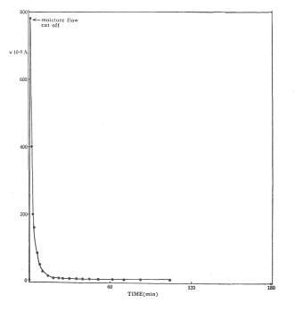
Fig. 12 Surface conductivty changes when moisture flow was cut off at the time of the peak. (mica)
