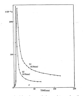
Fig. 3 Surface conductivity changes during moisture adsorption. (soda lime glass)
