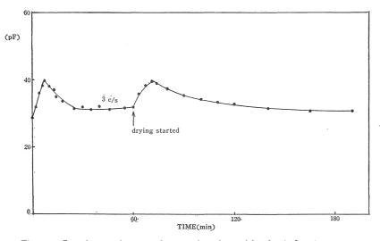
Fig. 11 Capacitance changes when a mica plate with adsorbed water was slowly dried. (mica)
