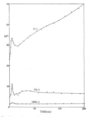
Fig. 22 Capacitance changes during moisture adsorption measured at the frequencies indicated, (filter paper)
