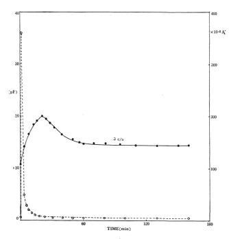
Fig. 5 The result of a simultaneous measurement of the capacitance and conductivity. (soda lime glass) Solid curve : Capacitance, Broken curve : Conductivity.
