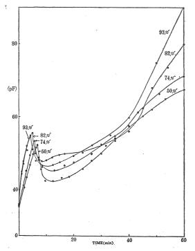
Fig. 20 Changes of capacitance at several relative humidities. (calcined diatomaceous earth)
