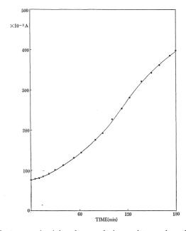
Fig. 9 Surface conductivity changes during moisture adsorption. (soda lime glass)
