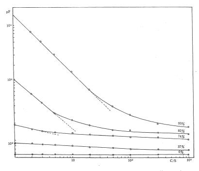
Fig. 7. The frequency dependence of the capacity of filter paper at various humidities (10 °C).
