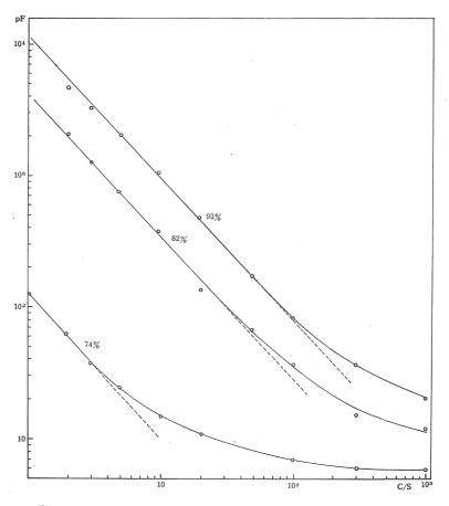
Fig. 1. The frequency dependence of the capacity of soda lime glass at various relative humidities (9°C).
