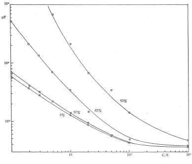
Fig. 4. The frequency dependence of the capacity of triglycine sulfate (b-cut plate) at various relative humidities (10 °C).
