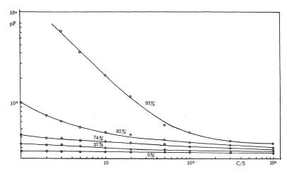
Fig. 5. The frequency dependence of the capacity of ceramic  $BaTio_3$  at various relative humidities (8°C).
