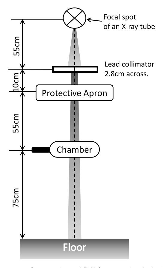
**Fig. 1** Geometry of an experimental field for measuring the lead-equivalent thicknesses and X-ray transmission rates of protective aprons.
