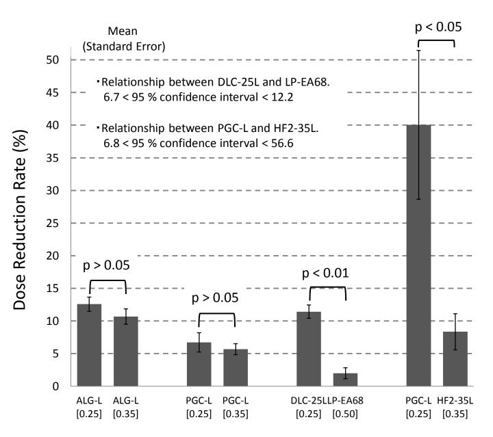
**Fig. 6** Difference in the dose reduction rate before and after the exchange of protective apron types in a practical field. '[ ]' in a figure expresses the lead-equivalent thicknesses of the X-ray protective aprons.
