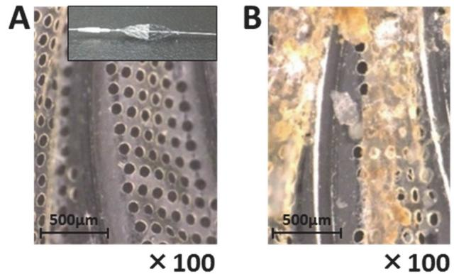
**Fig. 1.** View of the filter basket and internal side of the filter membrane of Filtrap<sup>®</sup> (NIPRO, Japan). A: Unused device, B: Membrane with the case of transient filter no-reflow. Note: a large amount of debris was observed.
