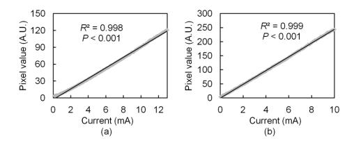
**Figure 6** Relationship between the signal intensity of NIR images and current (mA) in (a) 700 nm and (b) 810 nm LED. There was a high correlation between the signal intensity of NIR images and the current supplied to the LED at each wavelength. A.U.: arbitrary unit.
