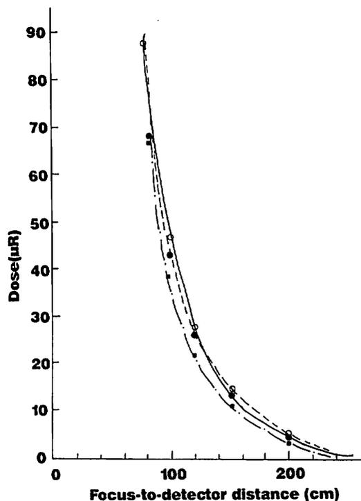
Fig 6: The relation between focus-to-detector distance and dose.
