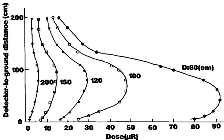
Fig 7: The relation between detector-to-ground distance and dose.
