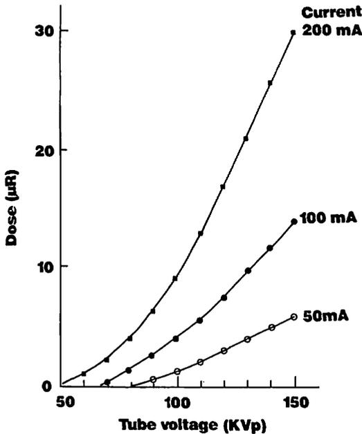
Fig 2: The relation between tube voltage and dose.
