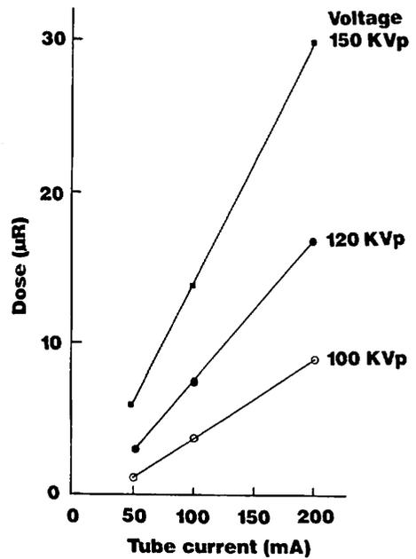
Fig 3: The relation between tube current and dose.
