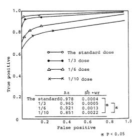
Fig. 8. ROC curves derived from the nodule detection test using FCR lower exposure images.
