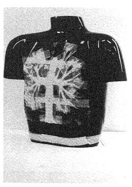
Fig. 2. Humanoid chest phantom with simulated pulmonary vascular vessels on its anterior surface.
