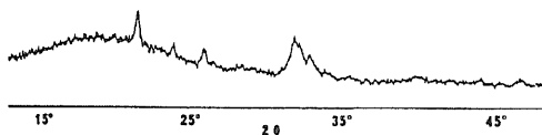
Fig. 11. The X-ray diffraction pattern of the crystals in a representative tumor coincides well with hydroxyapatite as illustrated in the JCPDS card.
