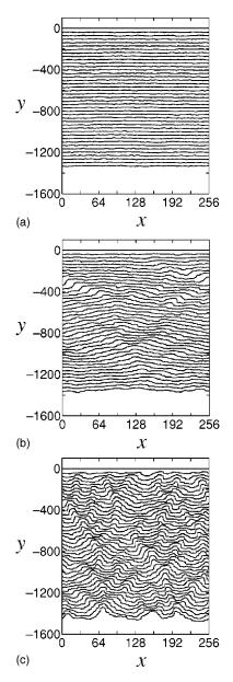
FIG. 2. Time evolution of the position of a perfectly permeable step in sublimation: (a) with the step-up drift (v = -0.1), (b) without the drift (v = 0), and (c) with the step-down drift (v = 0.1).
