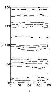
FIG. 9. A snapshot of the weak bunching of the impermeable step in sublimation at  $t=3.7\times10^4$ . The step distance is longer than the surface diffusion length, l=16 and  $x_s=8$ . The other parameters are  $A/k_BT=10$ ,  $c_{eq}=0.18$ , and  $\tilde{\beta}/k_BT=2.76$ .
