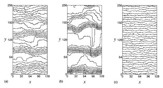
FIG. 13. Snapshots of impermeable steps in growth. The initial step distance is l=8, with  $x_s=16$ . Bunching (a) in the initial stage ( $t=1.9\times10^4$ ) and (b) in the late stage ( $t=3.1\times10^4$ ) with the step-down drift (v=0.2), and (c) a stable train with the step-up drift (v=-0.2) at  $t=3.1\times10^4$ .
