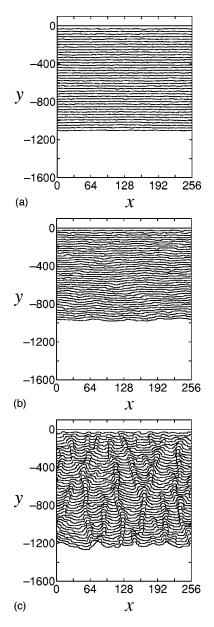
FIG. 5. Time evolution of the position of an impermeable step in sublimation (a) with the step-up drift (v = -0.2), (b) without the drift (v = 0), and (c) with the step-down drift (v = -0.2).
