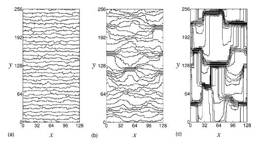
FIG. 7. Snapshots of impermeable steps with the repulsive interaction  $(A/k_BT=4)$  in sublimation: (a) stable  $(t=1.8\times10^4)$ , with the step-up drift (v=-0.4); (b) in the initial stage of bunching  $(t=1.0\times10^4)$ ; and (c) in the late stage  $(t=1.8\times10^4)$ , with the step-down drift (v=0.4).
