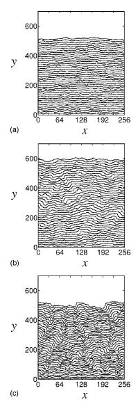
FIG. 10. Time evolution of the position of a permeable step in growth. The impingement rate is  $F = 2 \times 10^{-3}$ , (a) with the step-up drift (v = -0.2), (b) without the drift, and (c) with the step-down drift (v = 0.2).
