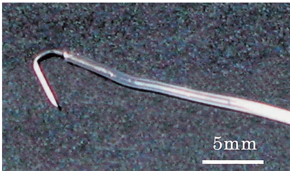
Fig. 1. A photograph showing the cannula using for blood samplings. The top of the cannula is connected with a syringe needle which is bent for insertion to the aortic bulb.
