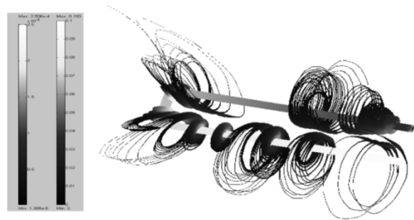
Fig. 4. Magnetic flux lines for meander sensor obtained from the FE model.
