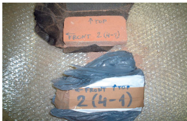
Fig. 10. An example of labeling of slice "2" (from the sample KSD 4-1, location "School"), which was distributed to labs in Japan.
